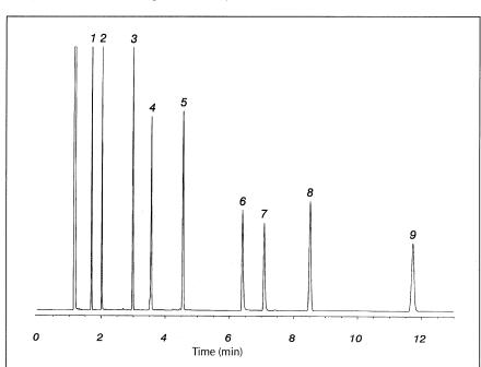
**Figure 1.** Chromatogram of a column test mixture. Conditions: column, DB-17, 30 m  $\times$  0.25-mm i.d., 0.15- $\mu$ m film; oven, 110°C isothermal; injector, split (1:75) (250°C); detector, FID (300°C); carrier gas, hydrogen (42 cm/s). Peaks: 1, undecane; 2, 1-octanol; 3, tridecane; 4, 2,4-dimethylphenol; 5, 2,6-dimethylaniline; 6, 1, undecanol; 7, ethyl decanoate; 8, 1-methylnaphthalene; 9, hexadecane.
